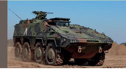
Adequate and timely re-supply is essential for a successful mission. BOXER Cargo variant is designed to transport and distribute two standard one tonne army pallets under armour to supply even exposed units on the battlefield.
