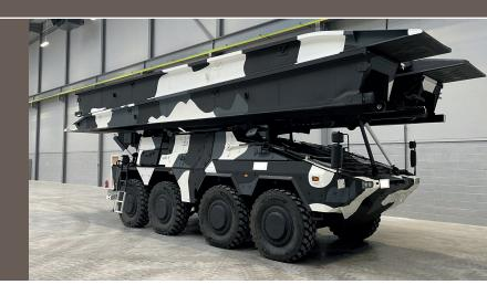
BOXER Bridge System combines the capabilities of the assault Bridge System Leguan with the unique protection and mobility of the combat proven wheeled armoured vehicle BOXER. This combination is the prerequisite for enforcement in high-intense conflicts, the provision of emergency temporary infrastructure during natural disasters and ensures flexibility for future military requirements and scenarios.
