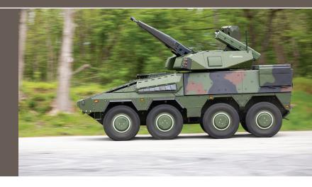
BOXER Oerlikon Skyranger® 30 (Skyranger 30) is a highly mobile air defence variant including active and passive search and tracking sensors and a powerful, autonomous shooter with both gun and missiles. It is capable of engaging modern battlefield threats with a special focus on small-unmanned aerial targets and combines superior firepower with the dynamics and elevation needed to successfully engage highly agile single or swarming targets performing loiter, pop up or dive attacks.
