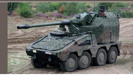
BOXER as Remote-Controlled Howitzer 155 mm (RCH155<sup>®</sup>) combines the firepower and effective range of the automated, remote-controlled Artillery Gun Module (AGM<sup>®</sup>) with the protection and mobility of the combat-proven wheeled armoured vehicle BOXER.
