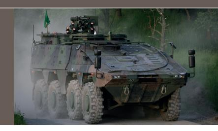
BOXER Armoured Engineer Group Vehicle (AEGV) is a troop and engineer group equipment carrier that enables the crew to execute tactical military and civil missions across the full spectrum of operations.
