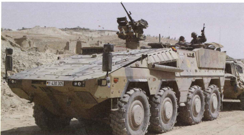
KMW has raised the remote weapon station on the Boxer A1 APC so that it can engage targets close to the vehicle. (Photo: Bundeswehr)
