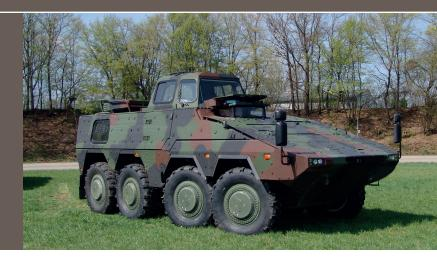
BOXER Driver Training Vehicle (DTV) provides realistic training for drivers of all BOXER variants and it permits the highest level of quality and safety of driver training. This variant consists of a standard Drive Module and the Driver Training Mission Module. Weight and ride behaviour completely match the characteristics of the Armoured Personnel Carrier (APC).
